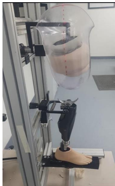
Figure 3.2 Transfemoral prosthesis with Genium knee joint during sagittal prosthesis assembly
