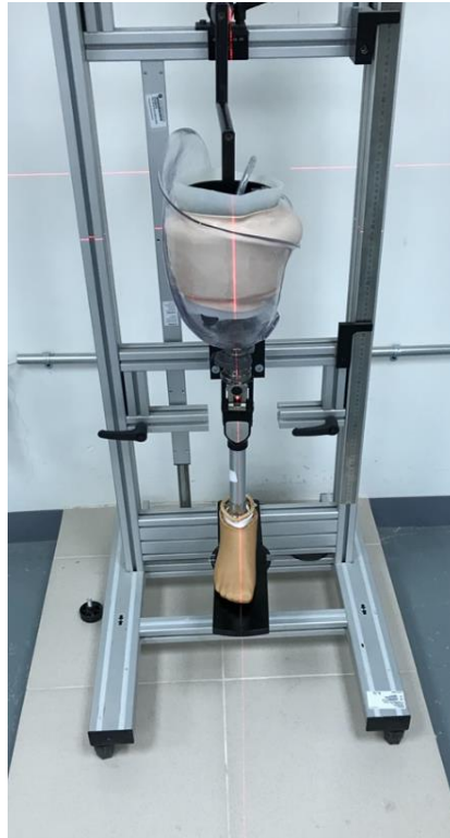
Figure 3.1. Transfemoral prosthesis with Total knee joint during frontal prosthesis assembly
